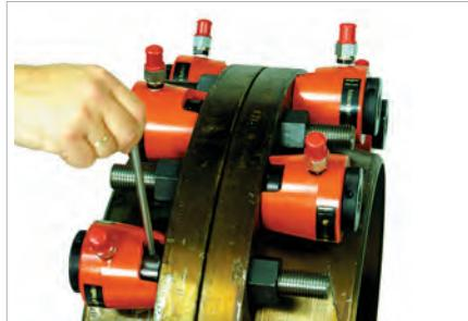
The tommy bar makes the nut socket (and therefore the nut) turn very easily
