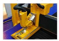
In case MSF Max is equipped with a laser bevel head, the system comes with the ACTG® unit and auto-calibration feature by default. Unlike in other MicroStep machines, the unit is integrated directly into the gantry in a combined calibration station that is ejected during the calibration process. The station contains also a pad for calibration of the capacitive height sensor in the cutting head and a nozzle cleaning system consisting of a camera and a wiping brush.
