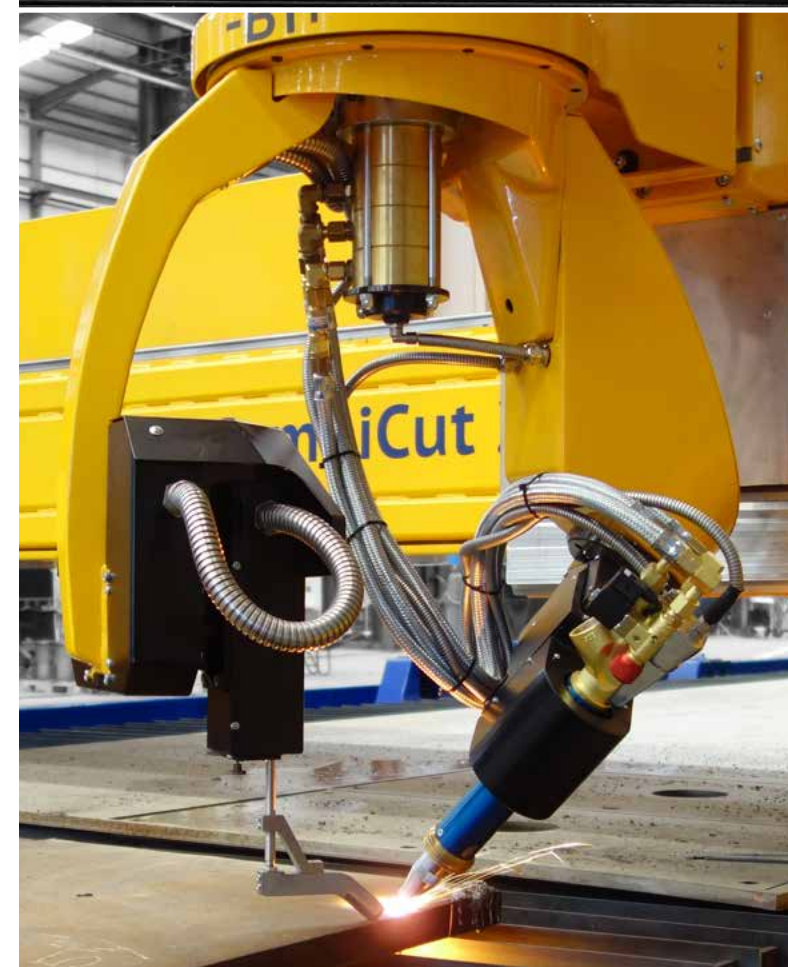
Bevel cutting with oxyfuel rotator
