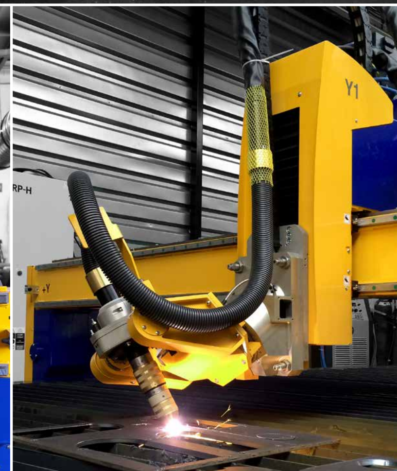
Active anti-collision protection for high safety standards
