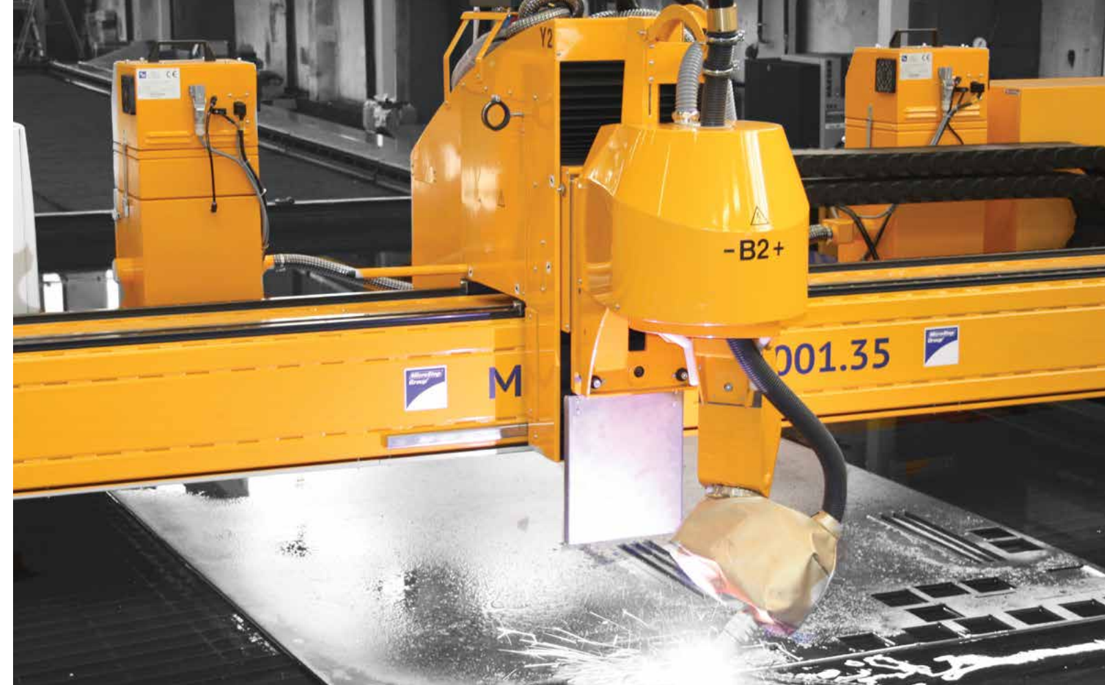
Plasma rotator performing bevel cutting on a water table
