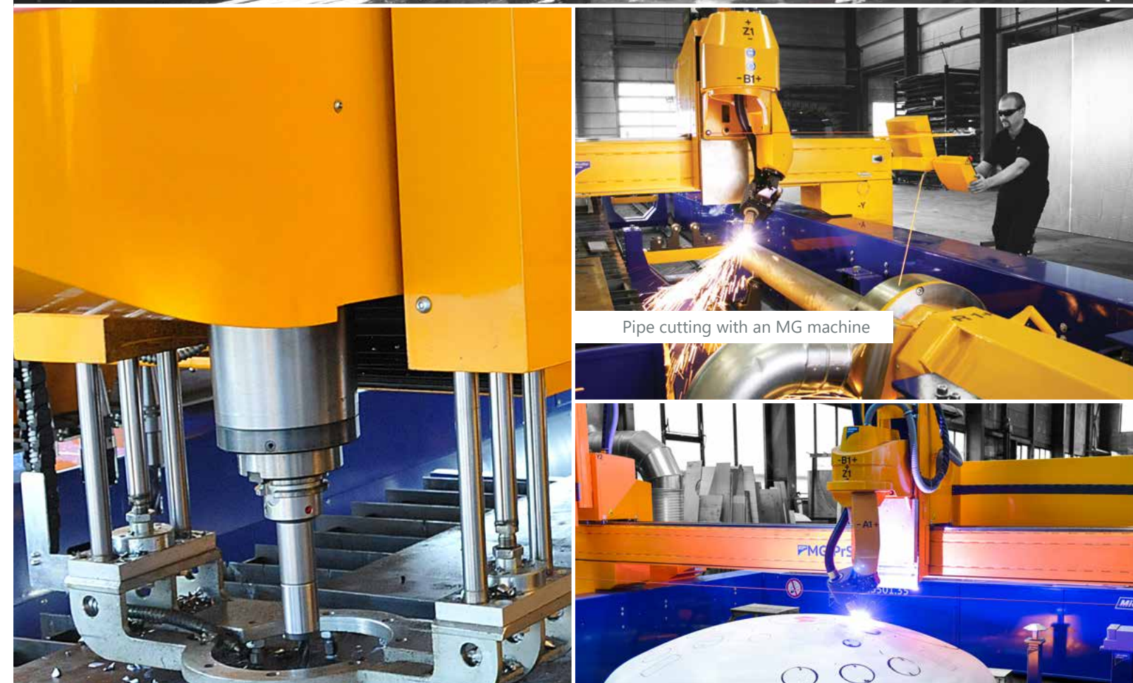
Dome processing with a multi-functional MG cutting machine
