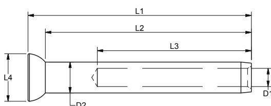
Blue Wave's ball terminals are marked with wire size and wire-hole depth to make it easier to work with and press or swage onto the wire.
