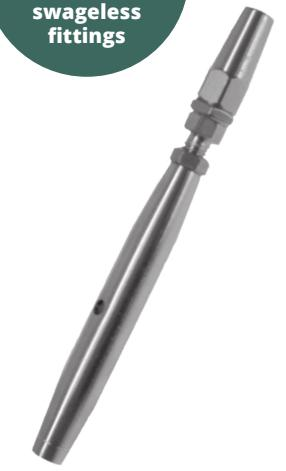
The "one side blank" rigging screw is assembled with a right threaded swageless terminal. It is ideal for site work where a professional swaging would normally be required and the final attachment has not been decided upon as the choice of fitting for the blank side is optional. See instructions page 14.
