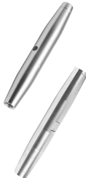
Blue Wave rigging screws bodies feature thread size, "easy use" marking for left and right threaded side and adjustment hole. From M20 upwards the bodies are available with chrome bronze threaded inserts and spanner flat on body for smooth adjustment.
