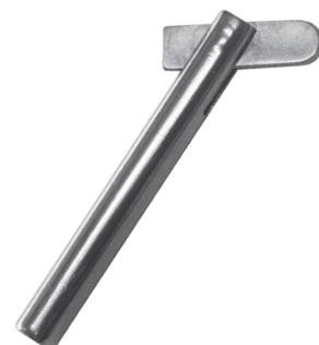
The dropnose terminal is e.g. perfect for tube handrails with vertical wire suspensions. Almost the easiest mounting imaginable - after being attached to the wire, drill a hole and stick through the drop nose end of the terminal and let it drop.
