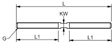
The opposite rigging screw would be a combination of the double threaded pin and inside threaded terminals locked at either side. This is usually used where extra adjustment lengths are needed or when pre-fitted wires are manufactured too short.
