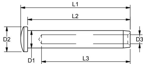
Domehead terminals by Blue Wave are engraved with wire size and swage depth marking, thereby making them easier to work with and to press or swage onto the wire.
