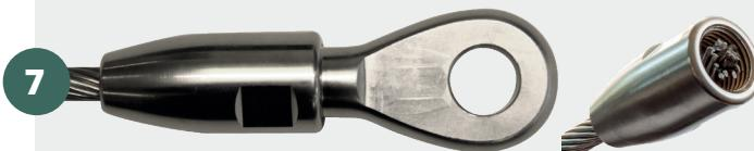
As a precaution take the terminal apart and visually check that the strands lay evenly around the cone and fit into the wire former (top part). Finally re-assemble as above and allow the Loctite to dry.
