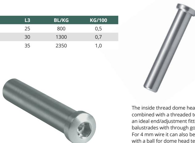
The inside thread dome head is, when combined with a threaded terminal, an ideal end/adjustment fitting for balustrades with through going holes. For 4 mm wire it can also be combined with a ball for dome head terminal, for diagonal or angle tensioning. The dome head features an Allen key hole and minimum overall dimensions.
