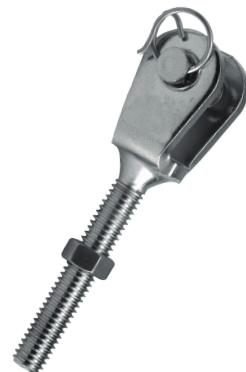
Small welded forks with thread and pin for the small rigging screw bodies, inside thread parts or other terminations. Available with left handed and right handed threads, incl. lock nut.
