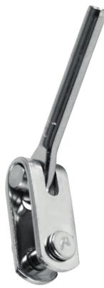
The flexible Blue Wave toggle terminal is marked with wire size and wire hole depth making it easier to work with and to press or swage onto the wire. Its uses are for diagonal or angle installations and also to minimize the risk of fatigue due to sideway loads.
