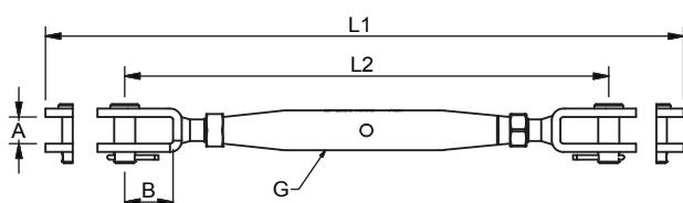
The larger size rigging screws from M20 and up are designed with a rounded fork head and are available with bronze threaded inserts for smooth adjustment.
