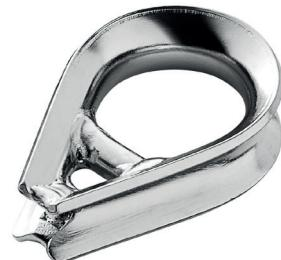
The reinforced thimble is based on the standard thimble but extra force is attained by the addition of a welded bar, as well as the ends of the thimbles being welded together.
