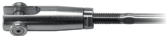
As an alternative to wire systems, tie bars are especially useful for static structures such as balcony supports and glass facade structures. Standard components include adjuster forks and inside threaded connectors. The tie bars are available on request and can be delivered with or without key width in a polished or unpolished finish. Adjuster eyes also available on request.
