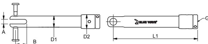
The one sized rigging screw is supplied with special lock nut and tamper proof press pins
