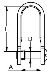
Note: All break loads are determined by pin and thread
