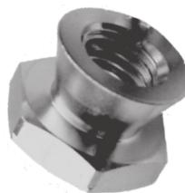
The security nut is the ideal solution where the nut has to remain permanently tightened. Once tightened, the KEY part breaks off and only a cone is left.
