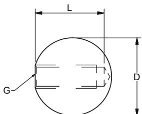
The range of WDS balls are used as stop ends to various wire fittings.
