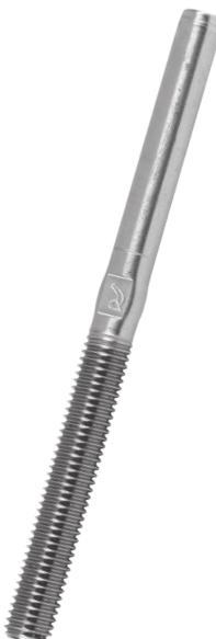
The wide range of threaded Blue Wave terminals are engraved with wire size and swage depth making them easy to use when pressing or swaging them onto the wire. The terminals are available with left handed or right handed threads and also with split pin hole or UNF thread on request. Threaded terminals are used to put tension on a wire either with the help of nuts and washers or as part of a rigging screw.
