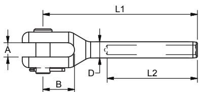
As demand for larger wire sizes has been growing, so has the range of larger machined fittings by Blue Wave. The machined forks are, as most fittings by Blue Wave, marked with wire size and swage depth marking for ease of use. From Ø28 mm wire/M48 forks are supplied with countersunk and double headed pins.
