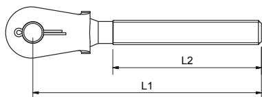
Welded forks with thread and pin for rigging screws, inside thread parts or other terminations. Available with left handed and right handed thread - also UNF sizes on request.
