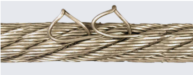
Protruded wires of inner rope
