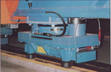
Roller Skate with a centre-plate, which is adapted to the diametre of the super-conducting coil.
