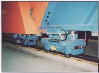
Roller Skates to solve the stocking and moving problems for the 3600 tonne experiments ZEUS and HERA.
