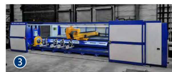
Combined MSF Pro machine for bevel cutting of plates up to 6 x 2 m and pipes up to 6 m length and Ø 300 mm diameter installed in Germany. Pipes and hollow sections are loaded manually from the side through the sliding side panels. The machine has a 6 kW laser source with beam shaping technology.
