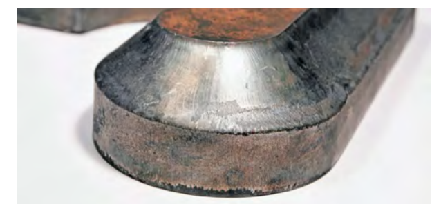
Close-up view of a cut part with added bevels.
