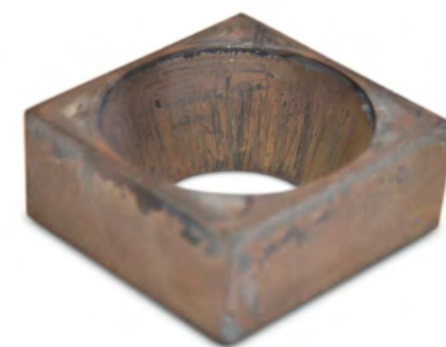
The leading Spanish machine manufacturer Solintal took advantage of MicroStep's oxyfuel rotator and ABP in a big way: the needed steel parts of up to 160 mm thickness with complex bevels on non-linear contours that previously took 6 hours to produce are now ready in 45 minutes.
