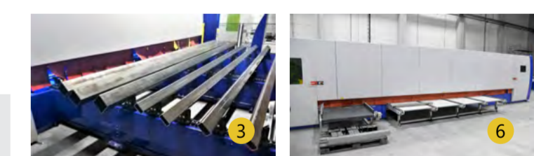
Automated pipe cutting machine MSF Pipe designed for 2D or 3D cutting of round pipes up to 6 m length and diameter Ø 200 mm as well as for tubes of rectangular and other cross-sections. The machine features a laser scanner that is used to determine the real shape of pipes to be cut to ensure accurate cutting results.
