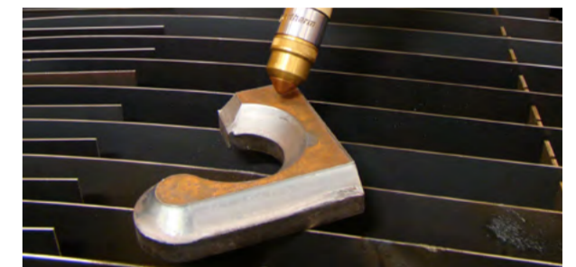
Thanks to high rigidity of the cutting machine, the cutting results are finer and more precise than with a robot.
