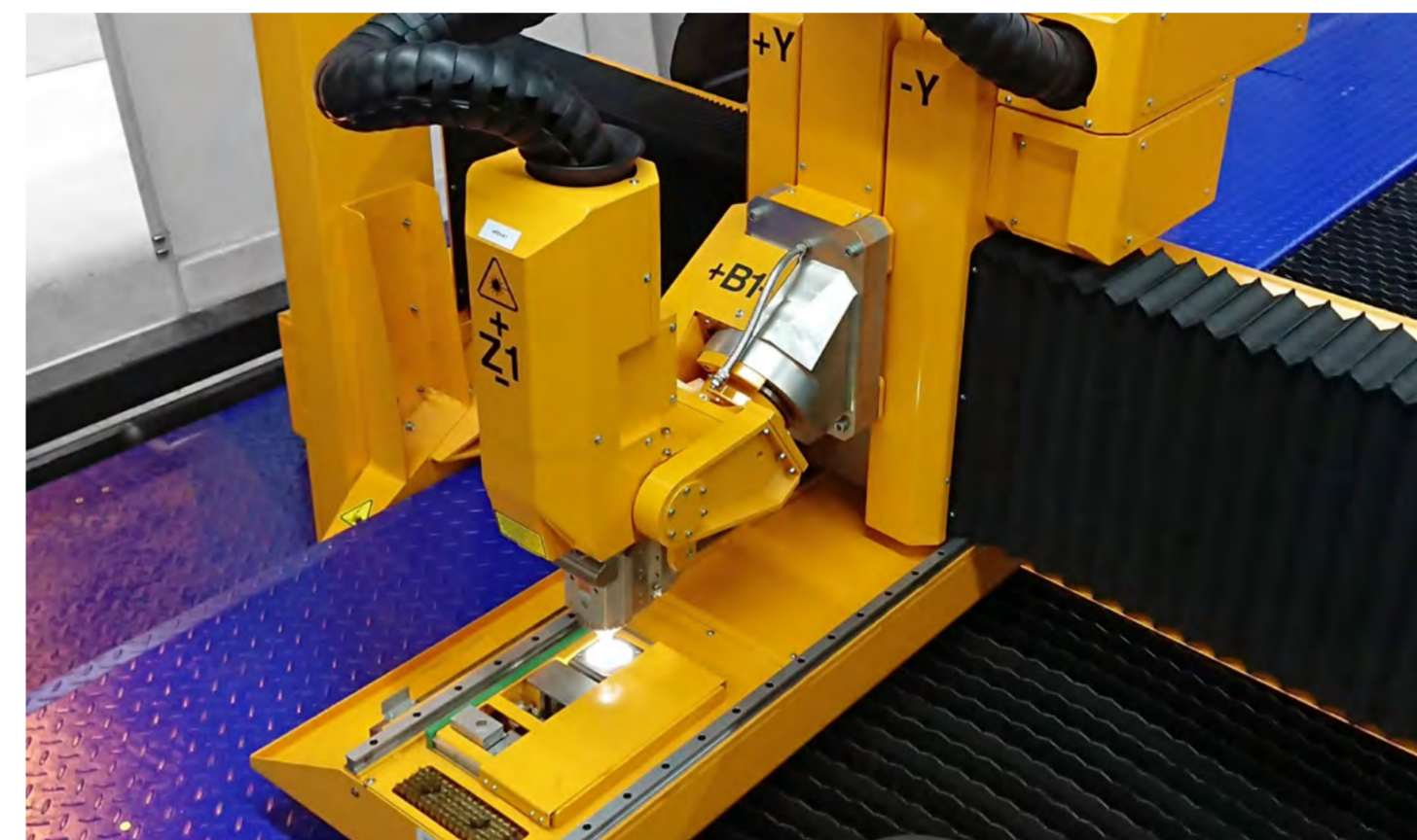
Above: Chantiers de l'Atlantique opted to invest into a large-scale fiber laser cutter MSF Max. It is a 50 m long machine with two 21,000 x 3,500 mm cutting zones.
