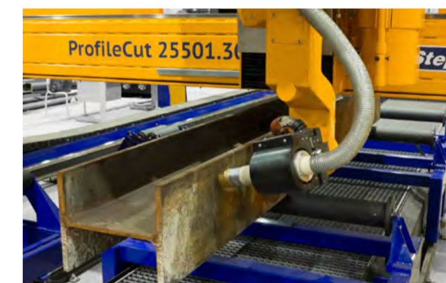
MicroStep has developed a variety of solutions for high-precision 3D processing of tubes, profiles and beams – including fully automated material handling.
