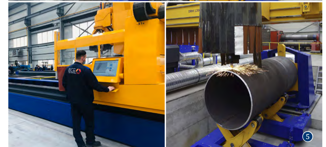
Plasma pipe cutting. The large positioner enables cutting of pipes up to Ø 2,000 mm, length 6 m and weight 7 tons.
