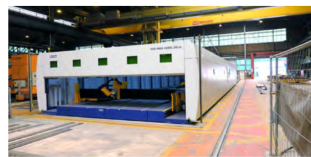
The machine is equipped with a bevel cutting head with 8 kW laser source that allows Chantiers de l'Atlantique to make weld edge preparation on parts up to 20 m long with thicknesses up to 16 mm and bevel angles up to 45°.
