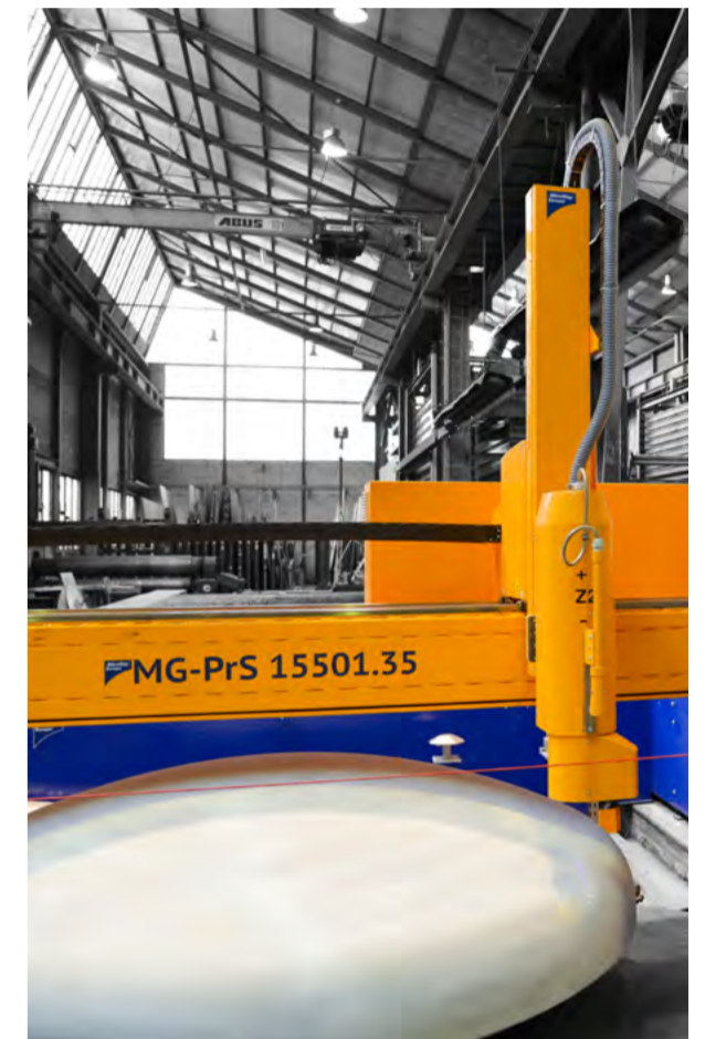
Thanks to the mScan technology, the 3D scan of a dome enables to determine production-related deviations from the ideal contour that then could be compensated for accordingly during cutting.
