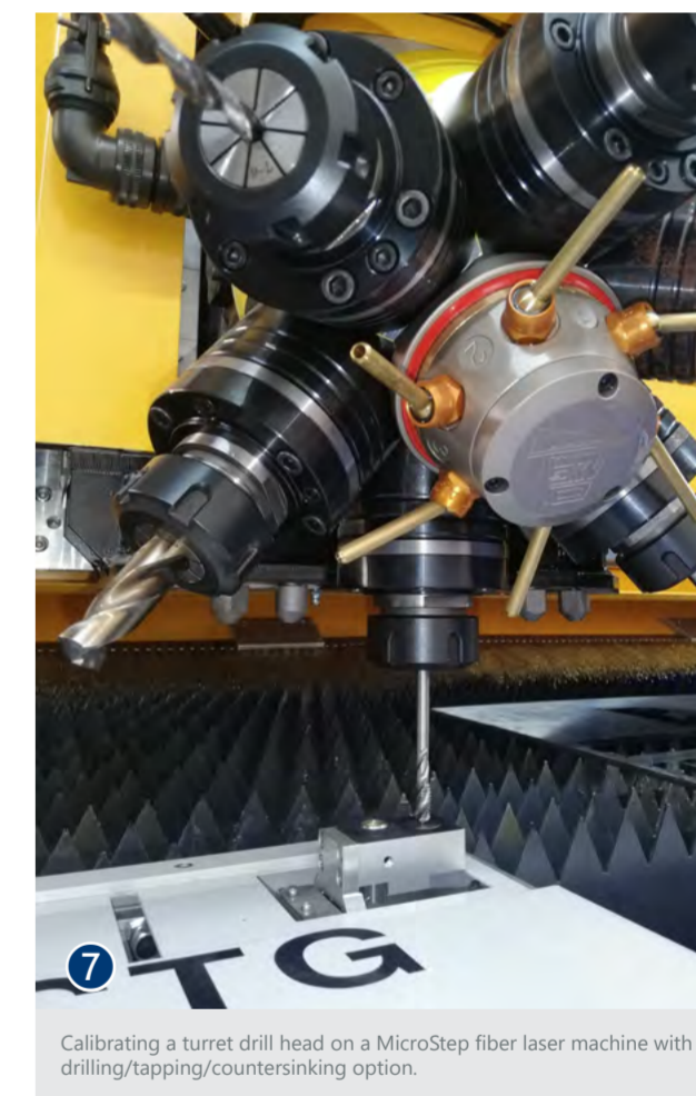
MicroStep drilling head with internal cooling and automatic tool change, with automatic tool magazines for 16 tools.
