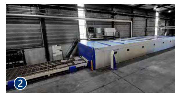
Large-scale fiber laser bevel machine MSF Pro with work area 16 x 3 m and a 15 kW laser source, installed at a Dutch customer.
