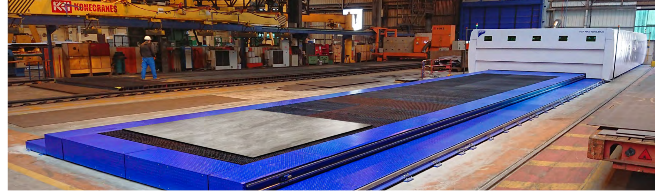
Above: Chantiers de l'Atlantique opted to invest into a large-scale fiber laser cutter MSF Max. It is a 50 m long machine with two 21,000 x 3,500 mm cutting zones.
