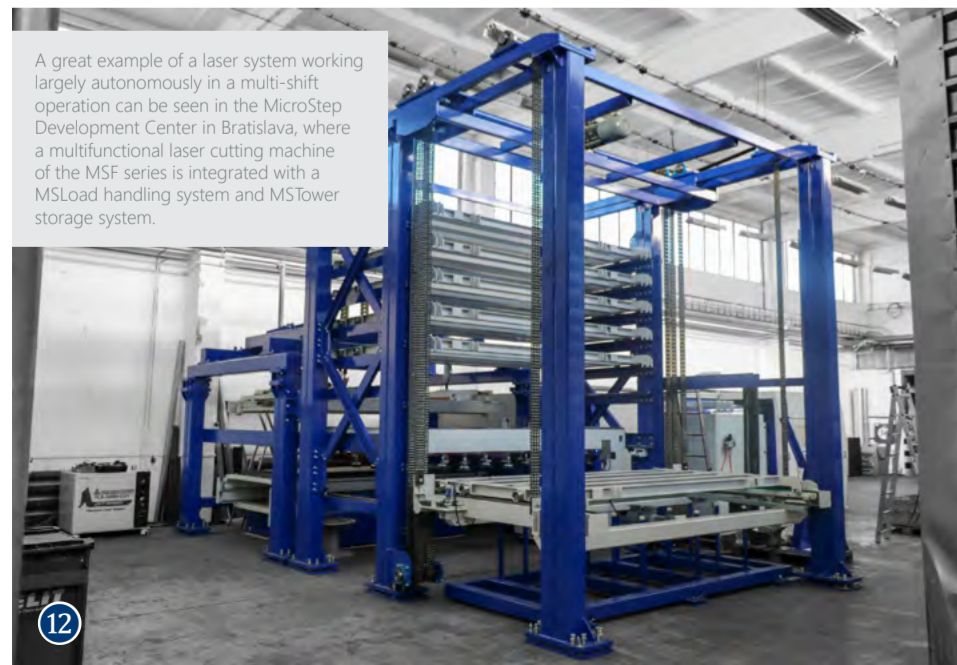
A solution used by one of the leading suppliers of industrial heating and cooling systems: a combination of the fully automatic loading system MSLoad with an additional conveyor, working together with a MSF laser cutting machine.
