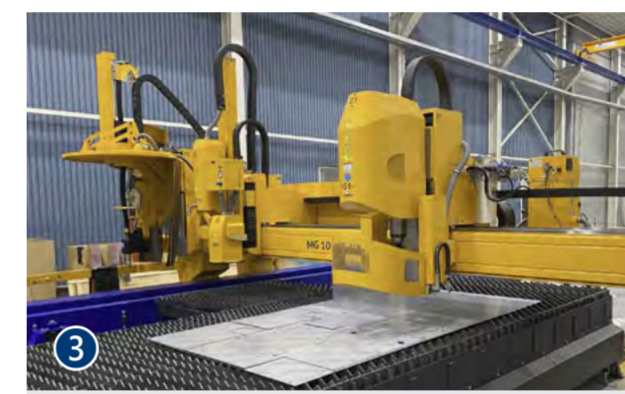
A multi-functional MicroStep machine with drilling up to Ø40 mm (+ tapping and countersinking), injet marking and a special plasma bevel head up to 120° tilt angle and endless rotation for plate, pipe beam and dome cutting.
