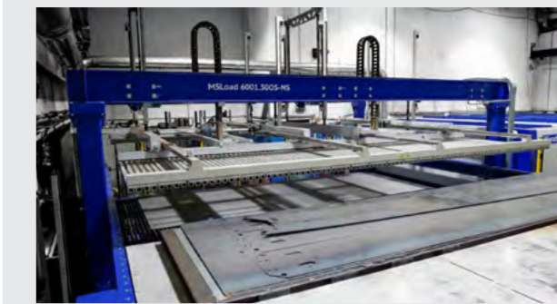
Unloading area of the middle pallet with MSLoad system, with a stockpile of unloaded orders in the front.
