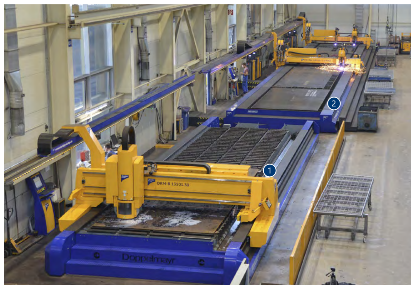
For the company Doppelmayr MicroStep installed a powerful drilling machine of the DRM series ① and two plasma and oxyfuel cutting machines of the MG series with two gantries ② + ③ each. The two MG machines are each equipped with a CCD camera ④ for maximum precision when cutting pre-drilled parts.
