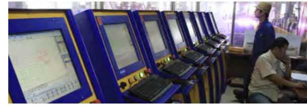
Operation 24/7: The automated cutting line (left) at ZMJ is controlled from a central control room (above). A total of eight CNC plasma cutting machines from MicroStep are automatically loaded and unloaded by a Demag process crane.
