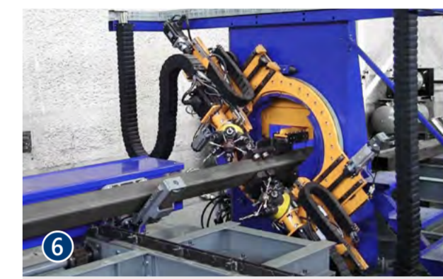
Profile drilling line DS-B allows simultaneous drilling, tapping and marking of rectangular hollow sections up to 12 m long and 300 mm wide.
