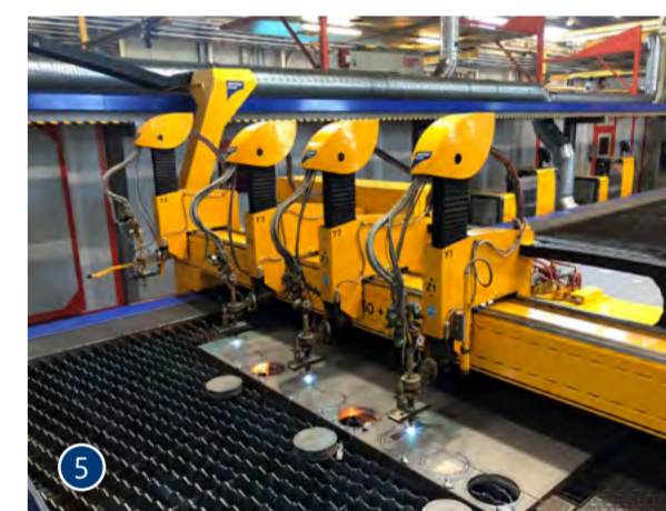
One of the four cutting gantries at Doppelmayr is equipped with four oxyfuel cutting heads for cutting of big material thicknesses. The more than 60-meter-long production line runs in three shifts at the headquarters of the company in Wolfurt (Austria) near the Bodensee Lake.
