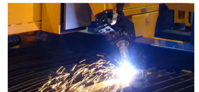
With beveling technology from MicroStep, V-, Y- and (under certain conditions) also X- and K-cuts can be added to already pre-cut parts.
