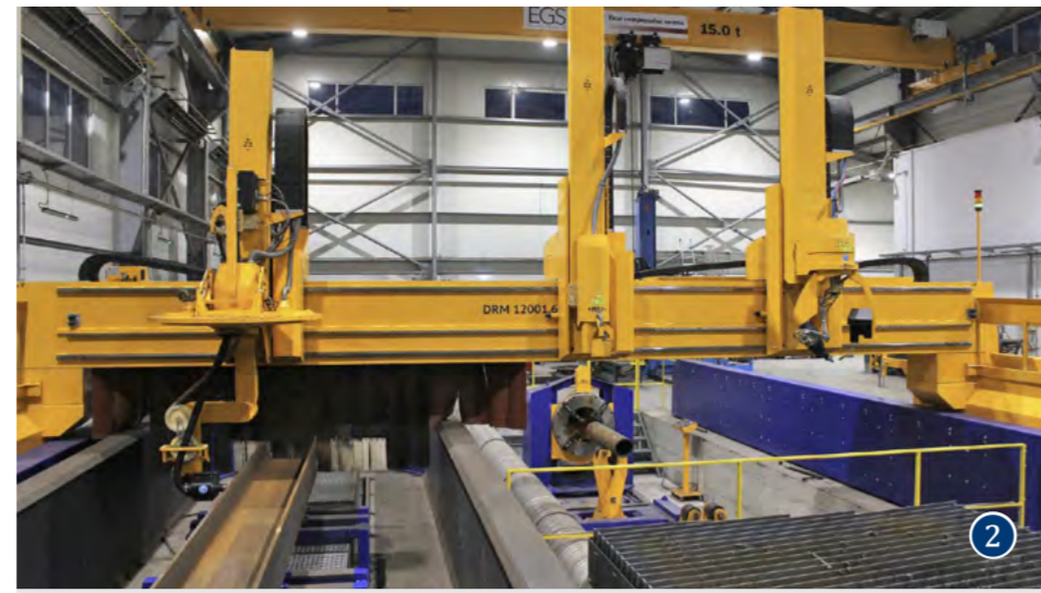
DRM gantry in EGS equipped with three tool stations. The machine has three work zones: cutting of beams (left), cutting of sheets and domes (front right) and cutting of pipes (rear right)
