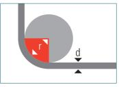
According to the German regulations for occupational insurance schemes [BGR] 500, Chap. 2.8, a sharp edge is already present when the edge radius 'r' is less than the material thickness 'd' of the lifting sling.
