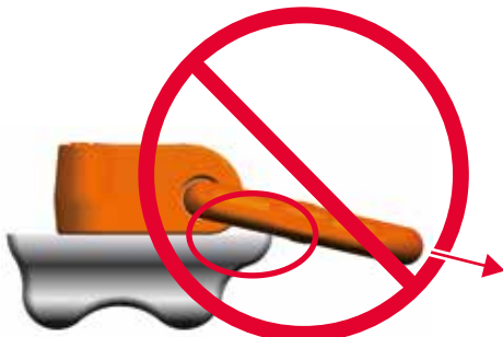
Improper loading as loading ring rests against edges or surfaces
