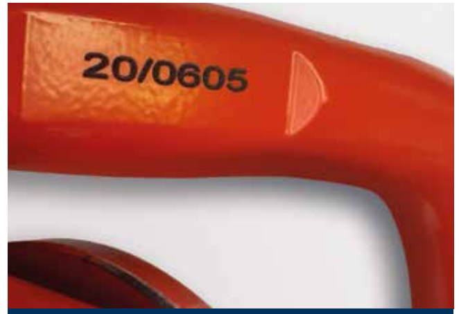
Laser engraved marking of the serial number
