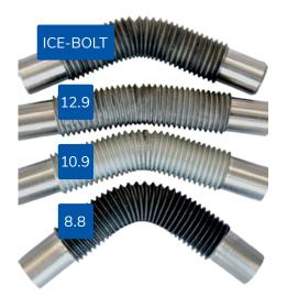
The thread of the ICE-Bolt proves itself in the prism bending test. The test shows: the ICE-Bolt masters static and dynamic WLL safely.
